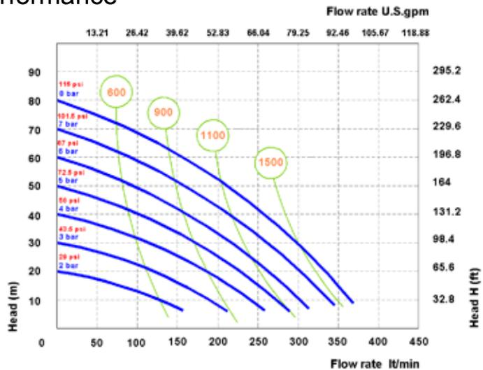
● Air supply pressure ● Air consumption Nlt/min
