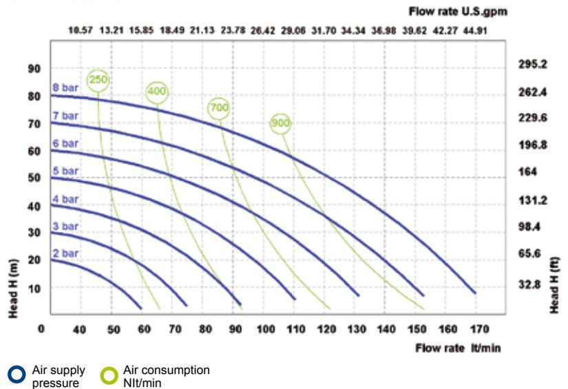
○ Air supply pressure    ○ Air consumption Nl/min
