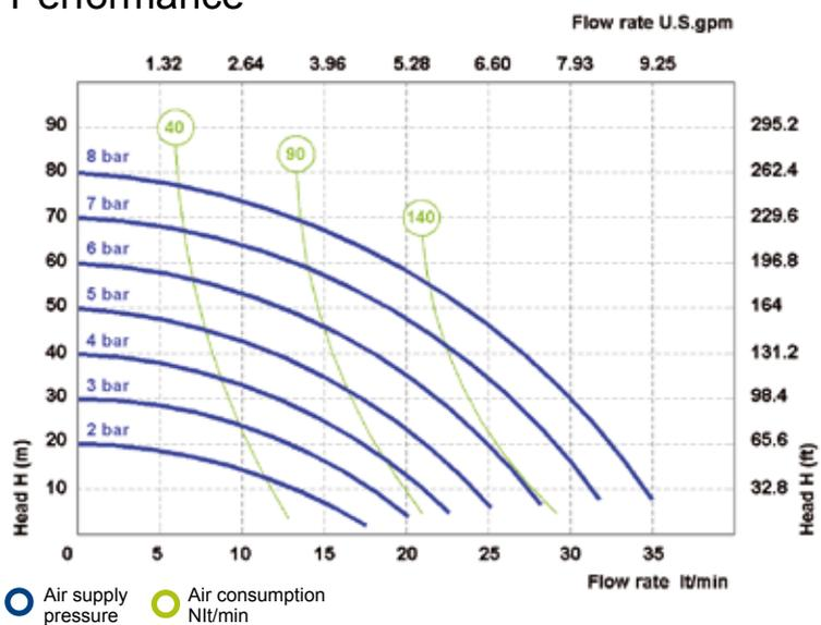
The curves and performance values refer to pumps with submerged suction and a free delivery outlet with water at 20°C, and vary according to the construction material.
