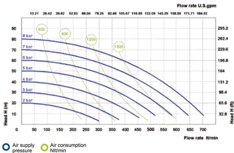
Air supply pressure Air consumption Nl/min
