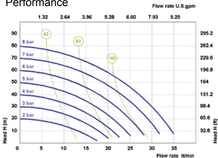
The curves and performance values refer to pumps with submerged suction and a free delivery outlet with water at 20°C, and vary according to the construction material.
