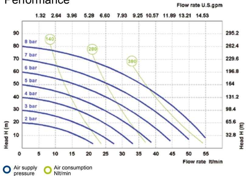
The curves and performance values refer to pumps with submerged suction and a free delivery outlet with water at 20°C, and vary according to the construction material.
