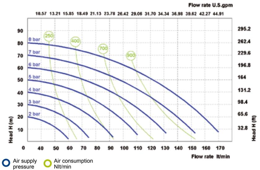
The curves and performance values refer to pumps with submerged suction and a free delivery outlet with water at 20°C, and vary according to the construction material.
