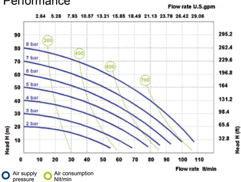
Air supply pressure Air consumption Nl/min
